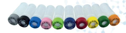
SEPARA® integrates in one single device auto-sampler vial, filtration membrane, plunger, and cap/septa.
