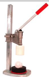
This press is specially made by Rowe Scientific to uniformly apply pressure to sample cups, reducing misalignment while maintaining film integrity.
