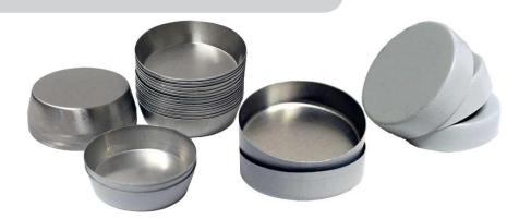
Australian made aluminium XRF pellet cups are available in the following sizes.
