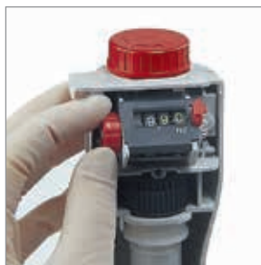
3. Pull the red knob and set the display to actual delivered volume (e.g., 9.90 ml).
