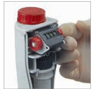
2. Lift gear lock lever to release.
