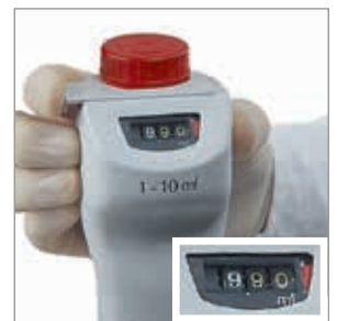
5. Replace housing – done! Alteration of factory setting is indicated by a red recalibration flag.
