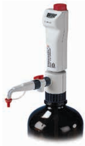
3. Pull the red knob and set the display to actual delivered volume (e.g., 9.90 ml).
