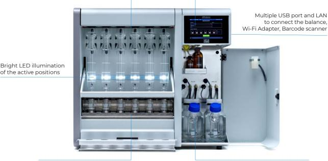
Advanced filtration system ensuring consistency and repeatabilty The trasparent tanks enable an immediate visualization of the reagents level
