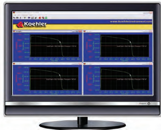
Real-time plot screen displays pressure versus time for up to twelve samples simultaneously.
