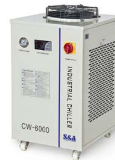
IC0716 - Chiller, Recirculating, 3015W Cooling Capacity, Digital Temperature Control, 13L/min Pump Outlet (12m Head) 15L Reservoir Tank 220V
