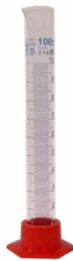
GC9005 - Cylinder Measuring Tall Form Spouted 100mL Glass with Orange Polypropylene Base
