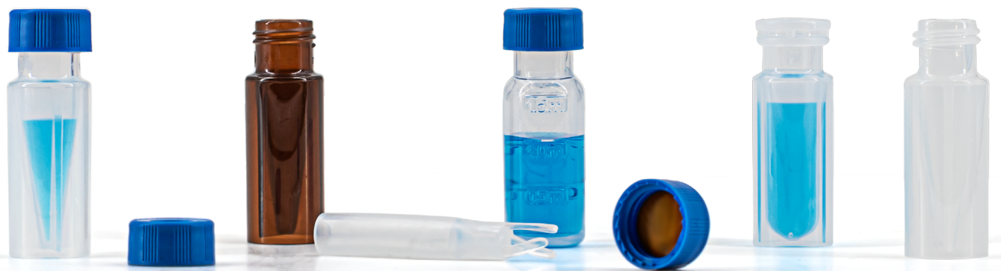
Figure 4: MACHEREY-NAGEL Polypropylene vials and fluorine-free closures for PFAS analysis
