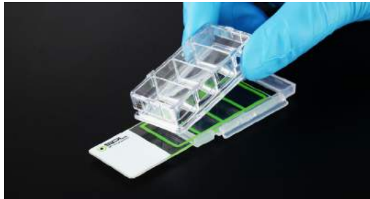
Cell Culture Slide I: Lean back both sides tabs and then chamber and holder will be removed from slide.
