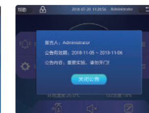
Announcement function designed for multiple persons to use the same incubator make clear to all users on important things
