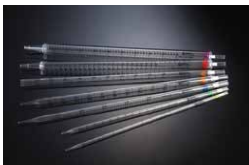
Serological pipettes (SPL), individual, sterile, DNase/RNase free, non cytotoxic, non pyrogenic
