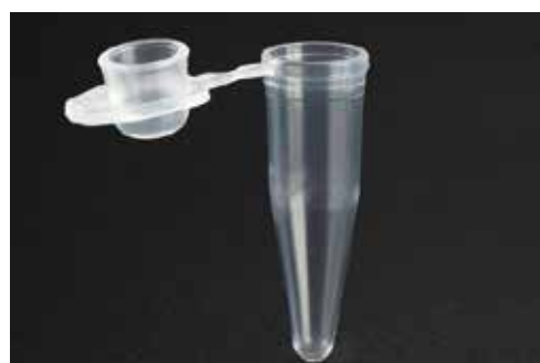
PCR tube (SPL), 0.2mL, single, dome cap, PP, 2 bags of 500. ROWE CODE PP0128
