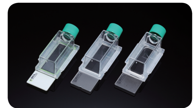
Cell Culture Slide II: Press chamber from top to bottom, then lean back and remove holder and chamber.
